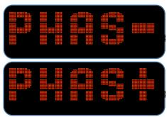
When the **MENU** key is pressed, the value switches between absolute polarity listening (PHASE+) and inverse absolute polarity listening (PHASE-).
