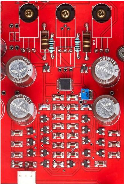
The design philosophy of the output stage for the **ZeroUno DAC-HPA** is very similar to the **CanEVER Audio LaScala PowerAmp**. The output stage is a Class A Single-ended Push Pull circuit with a high current audio line amplifier – capable of driving even low impedance headphones or in general, any heavy load as a power amplifier.
