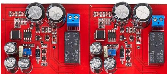
The output is protected against any DC current that might flow at the output in case of a fault. A double contact relay opens and protects the circuit, if needed.
