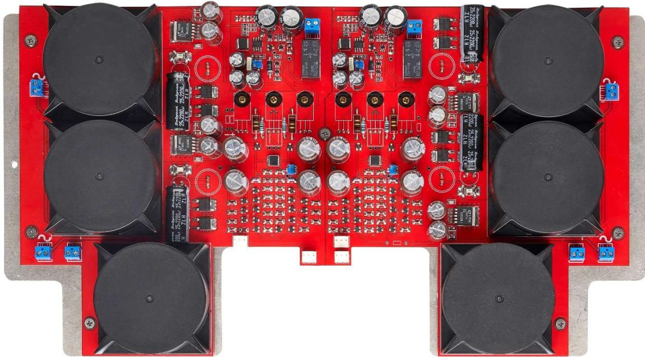
All the design ideas that made the *ZeroUno DAC* a well respected DAC, at the top level of performance in the market, are present inside the *ZeroUno DAC-HPA*, as well. The heart of the DAC board is an ESS Sabre<sup>32</sup> ES9018S chip, with its eight differential DACs used in a quad-sum configuration. The digital and analog filtering are a special design of *CanEVER Audio* and incorporate a dedicated output transformer topology inside the D/A interface.
