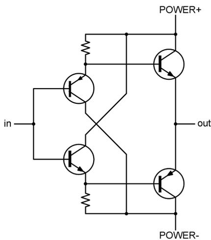
A lot of effort was spent to setup a super-linear circuit that overcomes the non-linearity problems of the above described circuit. The concept is based on the crossing of the driving signals, so that distortions will be naturally cancelled when summed at the push-pull driver in the output stage.
