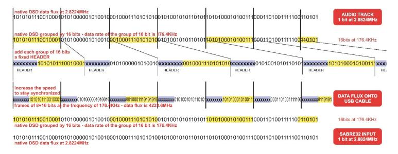
The "driver" (really CoreAudio for Mac OS and ASIO/WASAPI for Windows) has to collect 16 DSD bit, pack into a 24 bit *PCM* frame, and add the HEADER that it is always the same.
