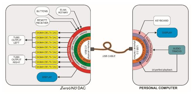
*DSD256* and *DSD512*, when there is a USB interconnection, cannot be managed as *DoP* so the only way to connect an equipment able of *DSD256* and/or *DSD512* is a dedicated custom driver able of *native DSD*.
