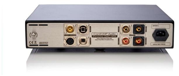
Input Connections:1xUSB, 1x SPDIF via RCA, 1x AES/EBU via XLR and 1x SPDIF via OPTICOutput Connection:2x Pairs of unbalanced RCA-Connectors: 1x Direct DAC Output and 1x PreampOutput,2x Pairs of unbalanced RCA-Connectors: 1x Direct DAC Output and 1x Preamp
