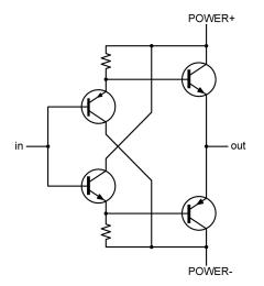
A lot of effort was spent to setup a super-linear circuit that overcomes the non-linearity problems of the above described circuit. The concept is based on the crossing of the driving signals, so that distortions will be naturally cancelled when summed at the push-pull driver in the output stage.
