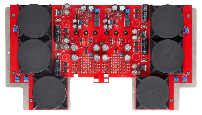
All the design ideas that made the **ZeroUno DAC** a well respected DAC, at the top level of performance in the market, are present inside the **ZeroUno DAC-HPA**, as well. The heart of the DAC board is an ESS Sabre<sup>32</sup> ES9018S chip, with its eight differential DACs used in a quad-sum configuration. The digital and analog filtering are a special design of **CanEVER Audio** and incorporate a dedicated output transformer topology inside the D/A interface.
