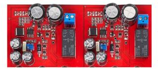
The output is protected against any DC current that might flow at the output in case of a fault. A double contact relay opens and protects the circuit, if needed.
