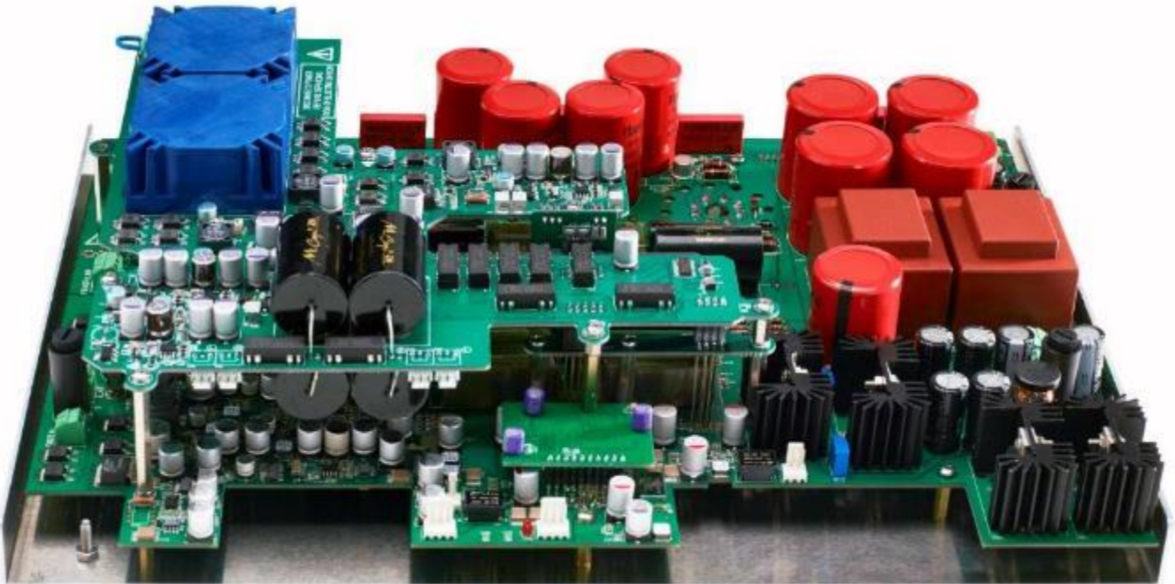
Fig. 1: The board with the Tube output stage, its power supplies and the DAC unit on the bottom and the board for the analog inputs mounted on top
