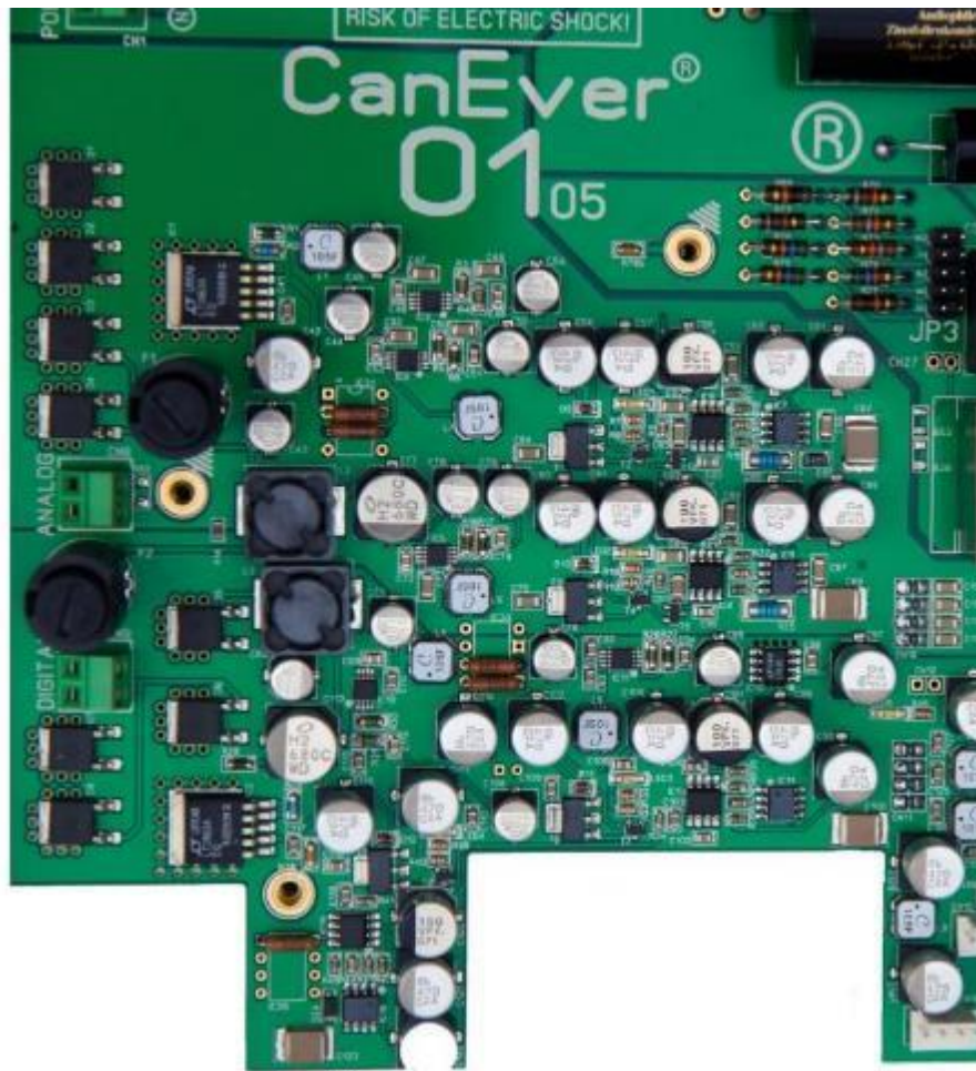
Fig.8: The discrete ultra-low noise power supplies in details
