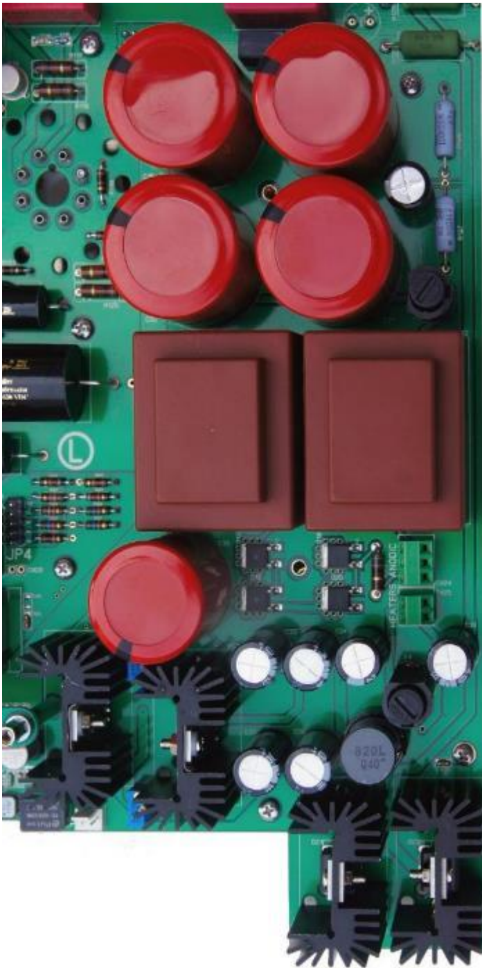
Fig. 7: The Tubes power supply – filament on the lower part of the PCB and for the anodic on the upper part
