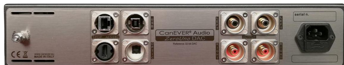
Fig. 7 The ZeroUno PURE DAC with the i2S input: SPDIF RCA, i2S HDMI, USB, OPTIC
