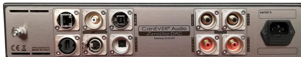
Fig. 8 The ZeroUno PURE DAC with the i2S input (optional configuration): i2S RJ45, i2S HDMI, USB, OPTIC
