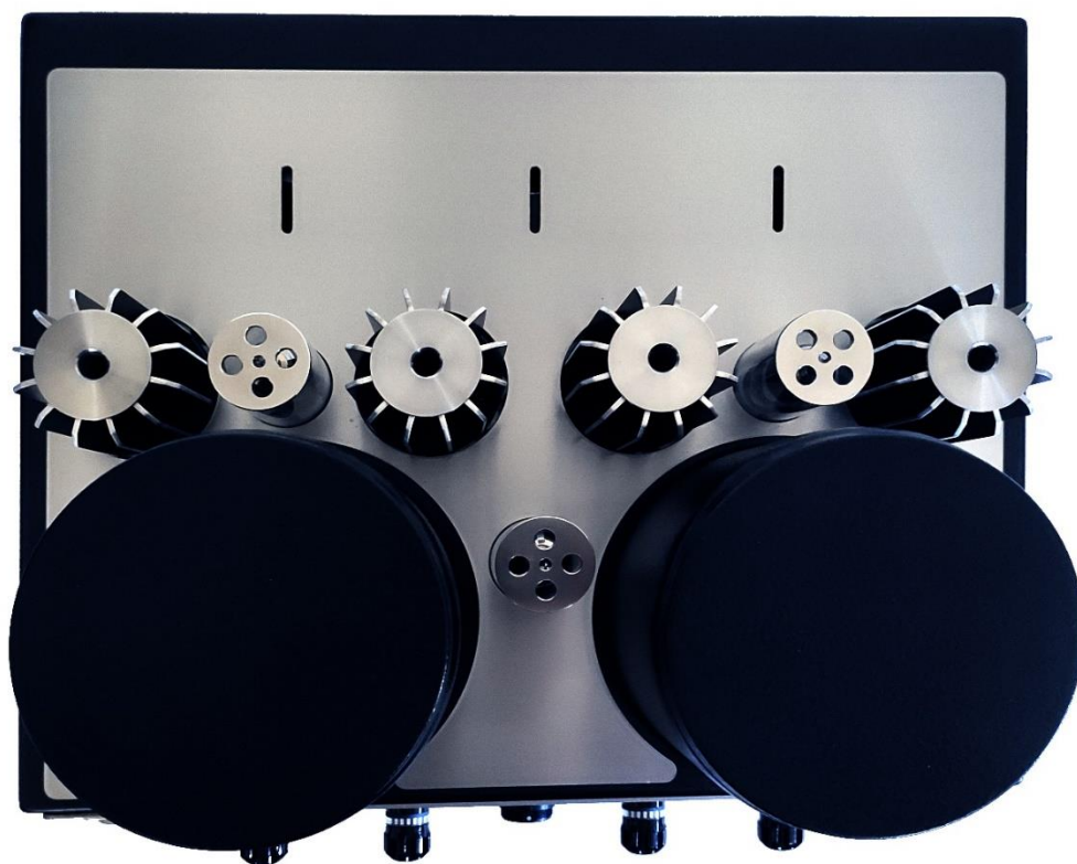
The driver stages between the daisy heatsinks The shunt regulator for the High Voltage Power Supply between the Output Transformer
