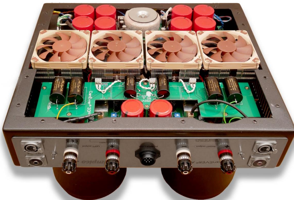
Fig. 15: The low speed Fans for the Air Circulation only The Olimpico PowerAmp can work without the fans
