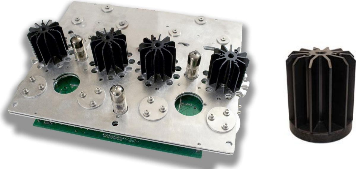
Fig.12: Heat Sinks on Top of the MOSFETs to cool the Olimpico PowerAmp
