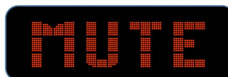
When the **MUTE** button is pressed, the *ZeroUno*<sub>SSD</sub> is muted and the display *never* switches back to the standard size view until the MUTE key is pressed again.
