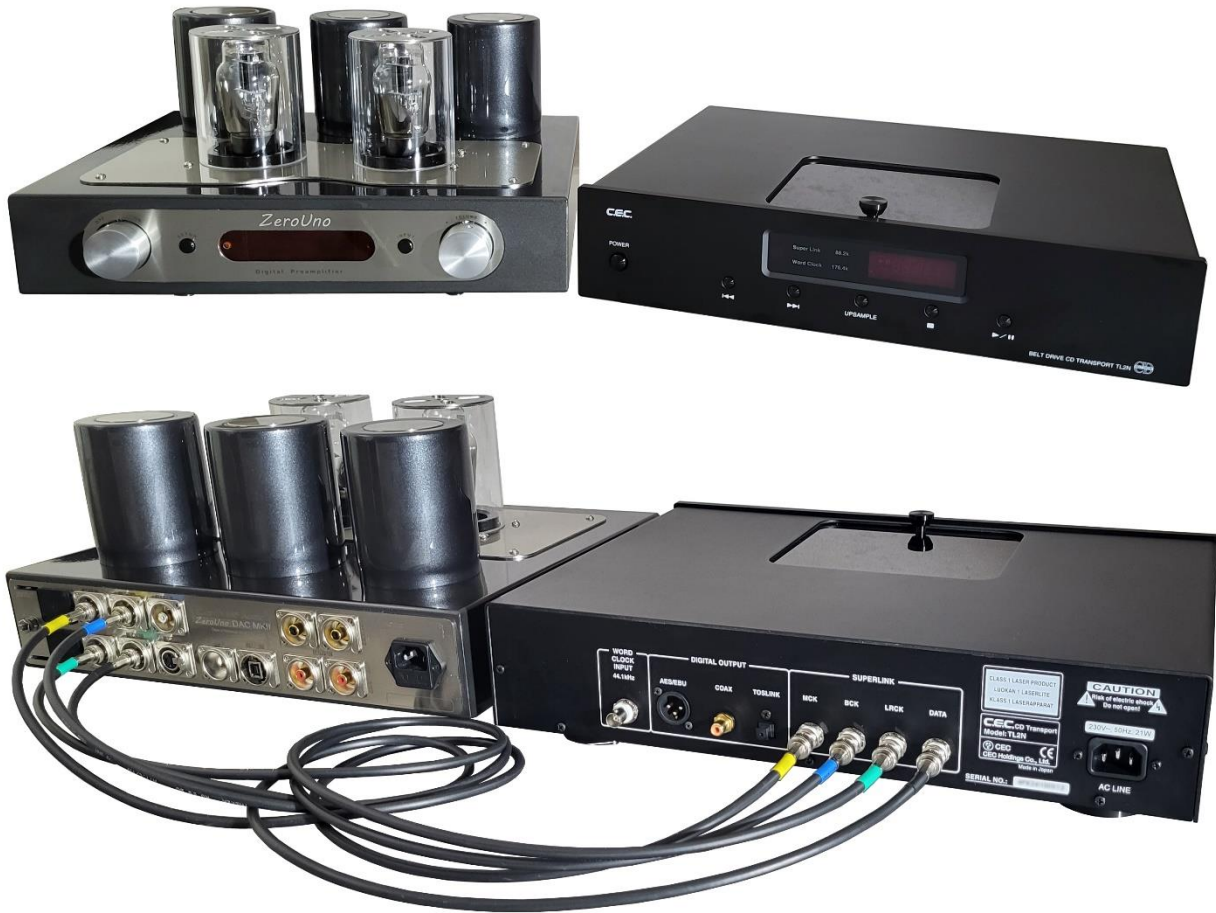
The ZeroUno DAC SE with the i2S capability custom configuration: i2S 4xBNC, SPDIF RCA, AES/EBU3, USB, OPTIC Connection to TL2N C.E.C. CD player
